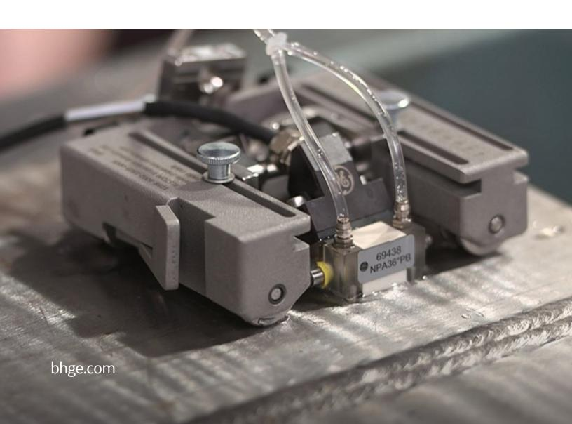
Weld inspections are crucial during the manufacturing process, as well as on a regular basis to ensure weld integrity. Inspections with conventional ultrasonic angle beam probes
