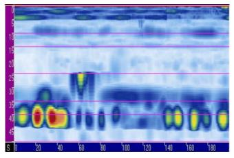
B-scan of weld displaying the depths of indications. The double V weld geometry of a 25 mm thick part is shown. Indications are detected between 1st and 2nd skip in the upper part of the weld at a depth of about 10 mm.
